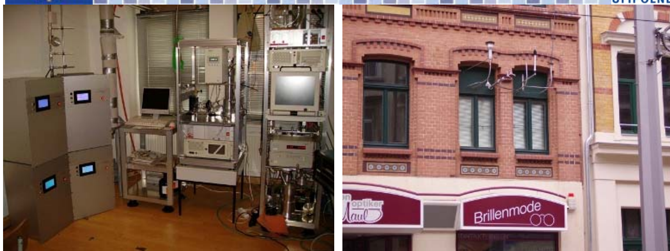
Fig. 3a, b Pictures of the 4 prototypes UFI 330 Sep-2006 at the IfT calibration test laboratory in the Eisenbahnstr. in Leipzig situated in a flat. High polluted ambient air in a street canyon is measured. (Photo: TOPAS)
