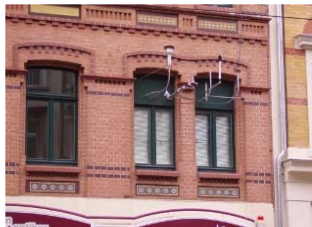
Pictures of the 4 prototypes UFI 330 in Sep-2006 at the IfT calibration test laboratory in the Eisenbahnstr. in Leipzig situated in a flat. High polluted ambient air in a street canyon is measured (Photos: TOPAS).
