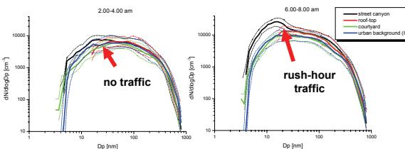
Median particle number size distributions for day times with low (left) and high traffic volume (right)
