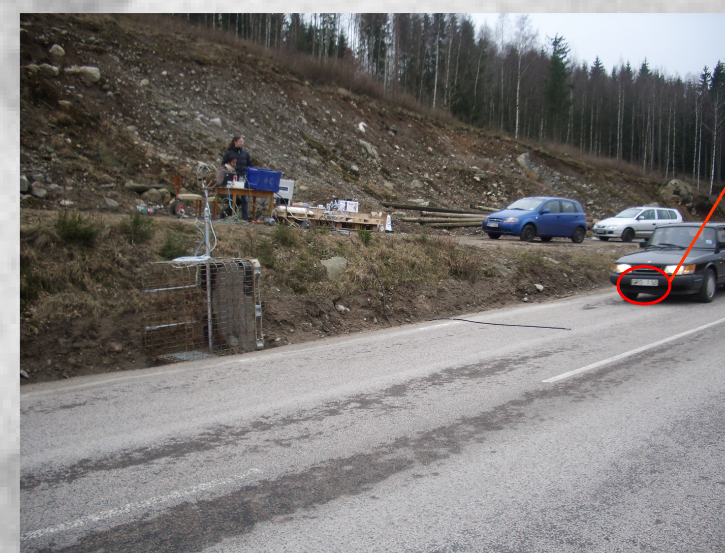
Figure 2 Car approaching the measurement site. Note the inlet tube in the centre of the near side lane.
