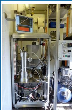
Appropriate instruments show particle number size distributions, which means they indicate how many particles of a defined size between 10 and 800 nm are in one cubic centimetre air at a certain time. The function of the instrument is based on charging particles, followed by segregation of particles in an electrical field according to their diameter and charge. In a last step, the classified particles are counted by a particle counter.
