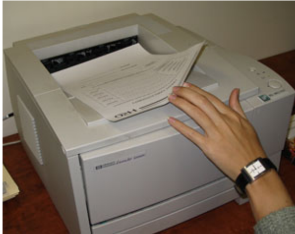
(Photo: Lidia Morawska) This printer in a Brisbane, Australia, office building contributed to higher particulate matter concentrations indoors than those outside near a freeway.
