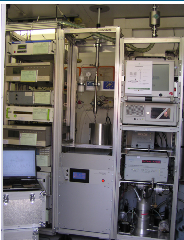
Fig. 2 Dresden: UFP 330, TOPAS (middle) and reference Twin-DMPS, IFT (right)
