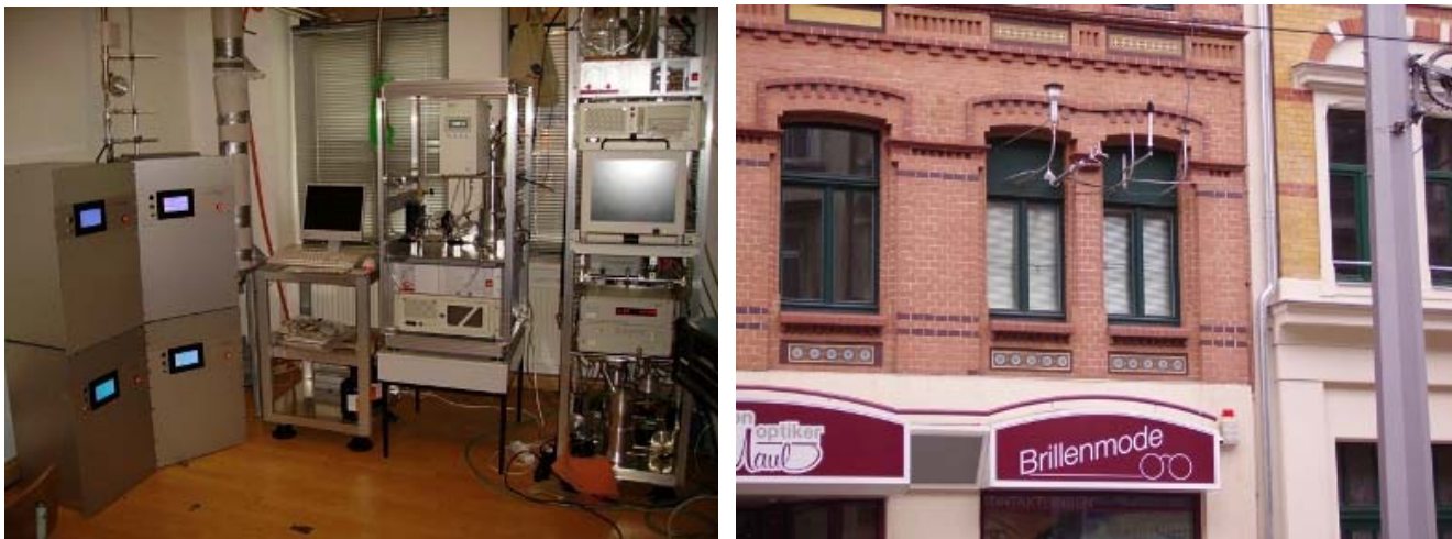
Fig. 5a, b Photos of the 4 prototypes UFP 330 Sep-2006 at the common IfT/ UfZ (Helmholtz Zentrum für Umweltforschung – UfZ) calibration test laboratory in the Eisenbahnstr. in Leipzig situated in a flat. High polluted ambient air of a street canyon was measured. (Photo: TOPAS)
