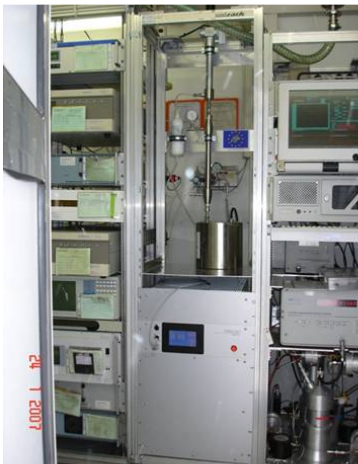
Fig. 3 UFP 330 at the pilot station Dresden Schlesischer Platz working since 21.12.2006 (Photo: L. Hillemann).
